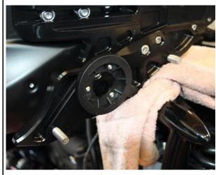
Using the screws provided, screw the receiver of the antitheft device (keyless antenna) onto the seat bracket from below (the original holder is obsolete).
