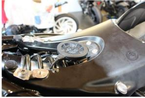
Loosen the receiver of the anti-theft device (keyless antenna).
