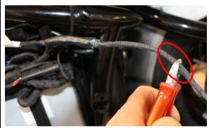
Cut the cable harness at a distance of approx. 20 cm from the connector.
