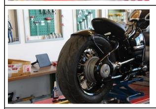
Remove the rear wheel again and tighten all fender screws.
