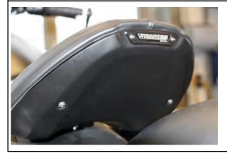
Attach the emblem using the two screws (M4) provided.
