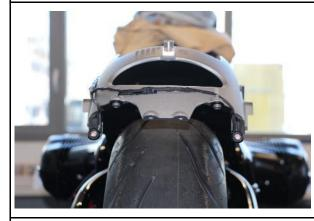
Completely remove the rear lighting.
