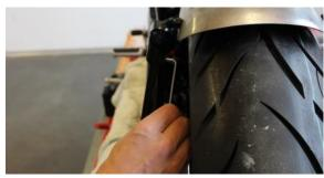
The thread pin on the inside of the rear lights can be used to align the fender and the rear lights.
