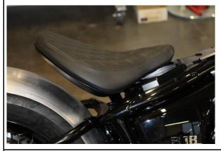
Attach the seat shell onto the holder using the two screws and large diameter washers provided, adjust as required and tighten.
