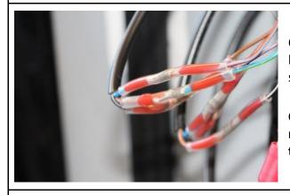
Connect both three-core cable to the original cable harness according to the diagram using the enclosed solder connector.
