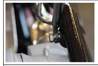
Attach the two braces to the swingarm using the screws and safety washers provided.
