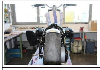
Remount and reattach the rear wheel, brake caliper and all removed parts.
