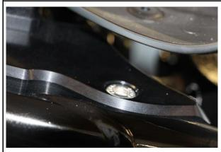
Attach the complete holder using the screws provided.
